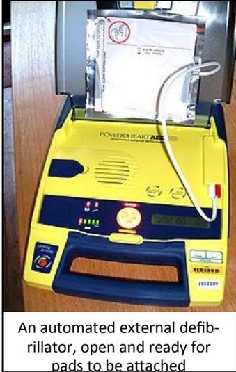
An automated external defibrillator, open and ready for pads to be attached
